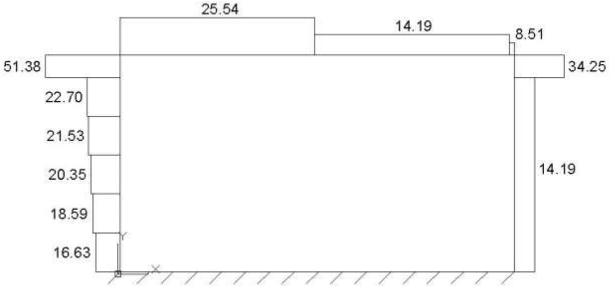
Figure 11: N-S Wind Pressure Diagram
