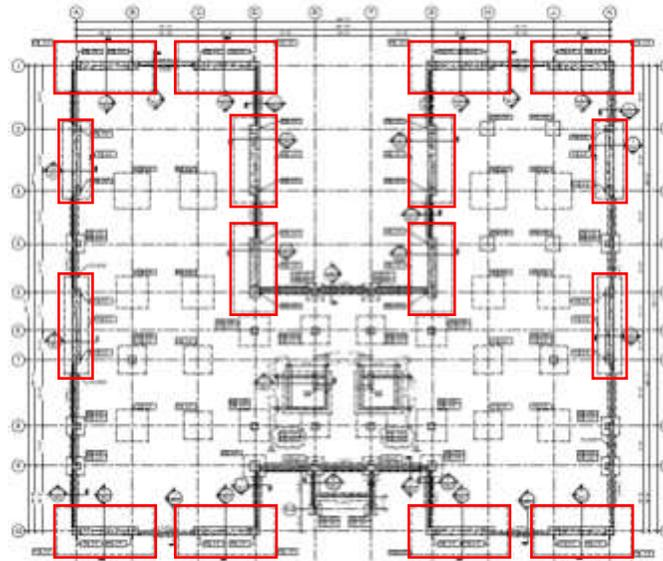
Figure 3: Braced Frames/Combined Footing Locations
