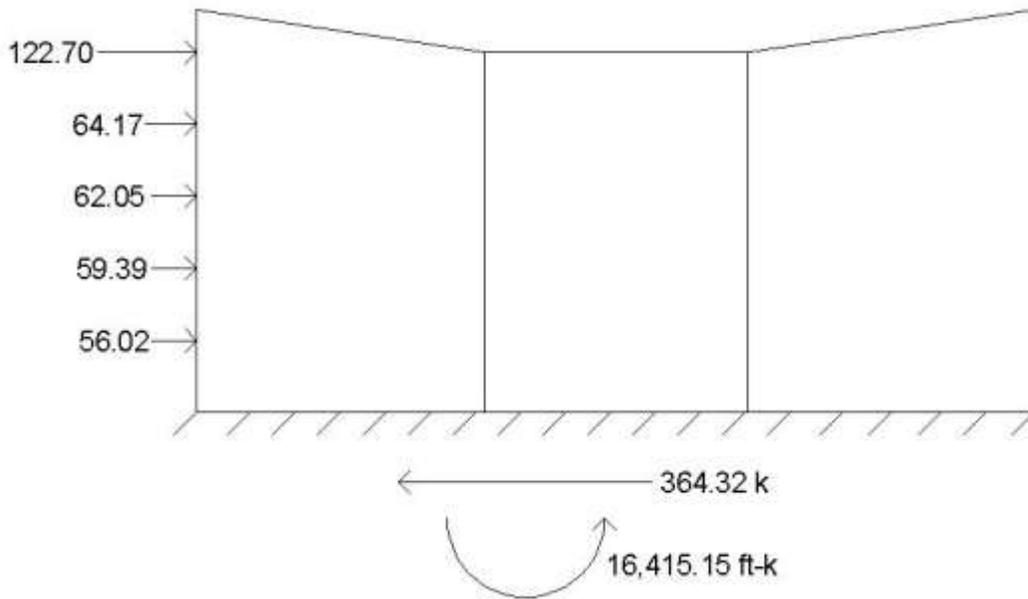
Figure 16: E-W Wind Force Diagram
