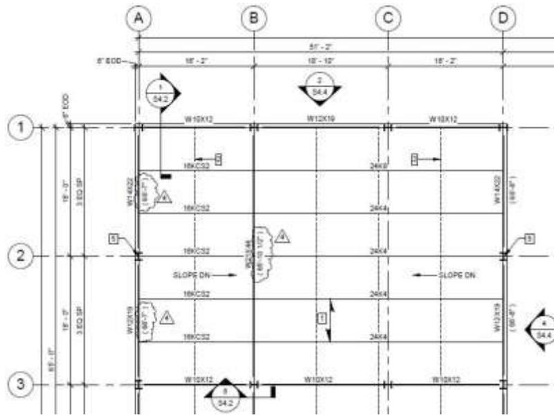
Figure 5: Typical Roof Framing Plan (Enlarged)
