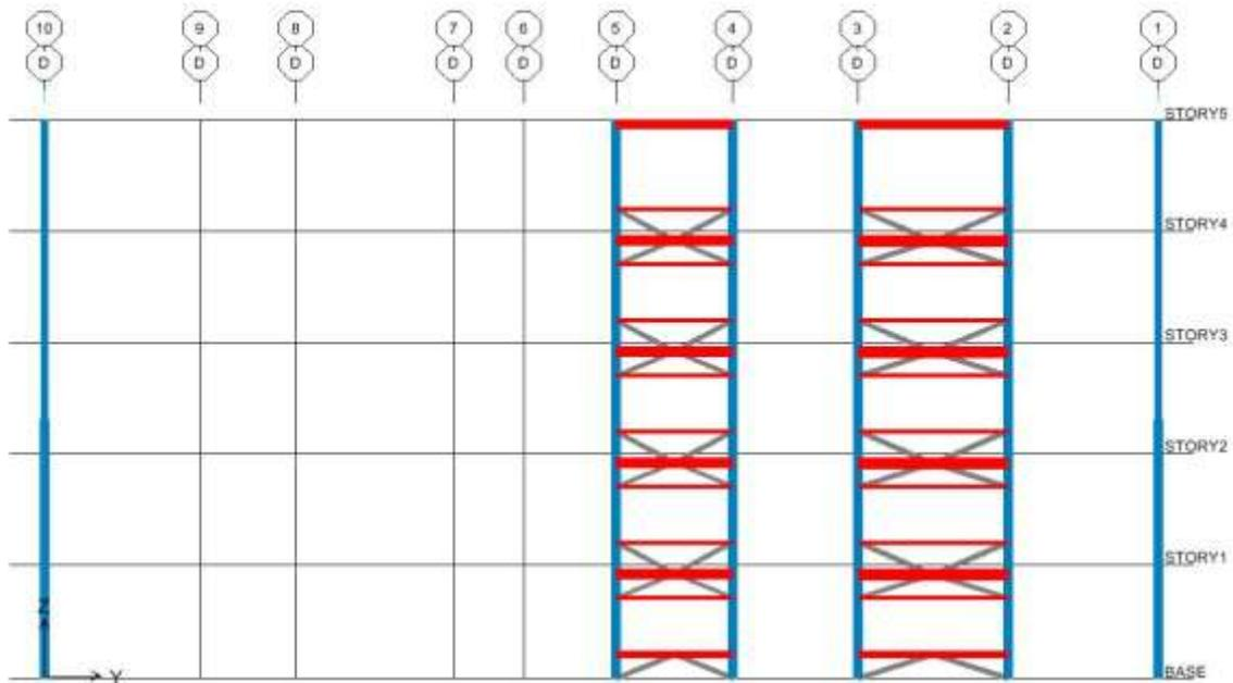
Figure 23: Braced Frames at Grids D and G
