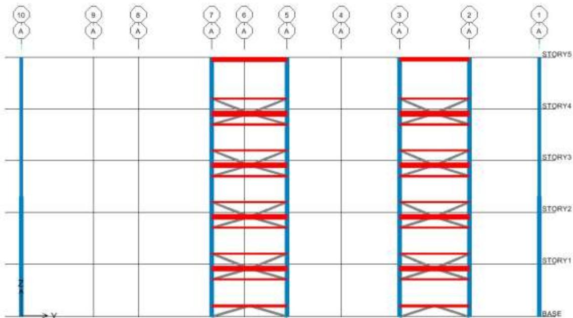
Figure 22: Braced Frames at Grids A and K
