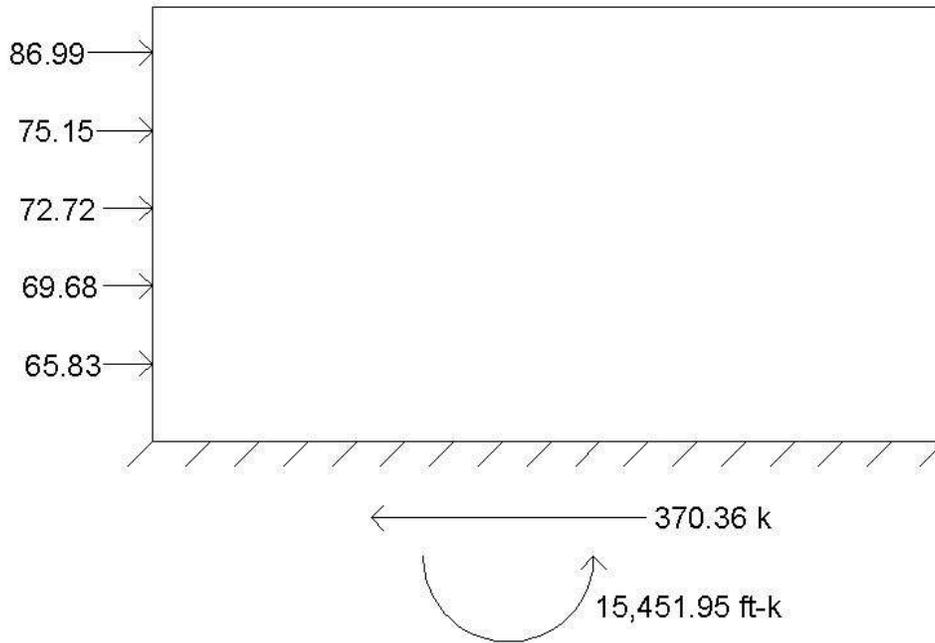
Figure 12: N-S Wind Force Diagram
