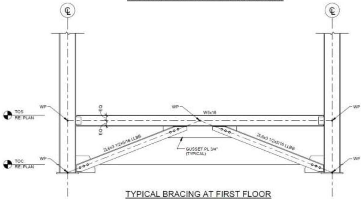
**TYPICAL BRACING AT FIRST FLOOR**
